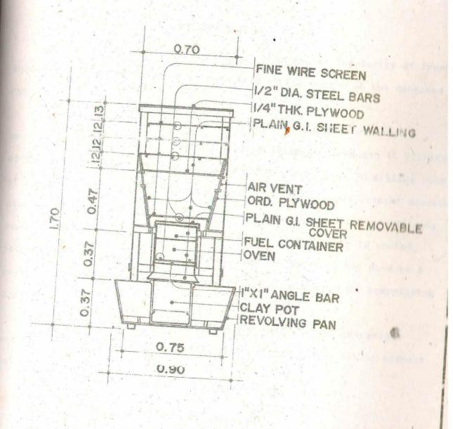
FIG. 7. TYPICAL CROSS SECTION Scale: 1:20 meter
