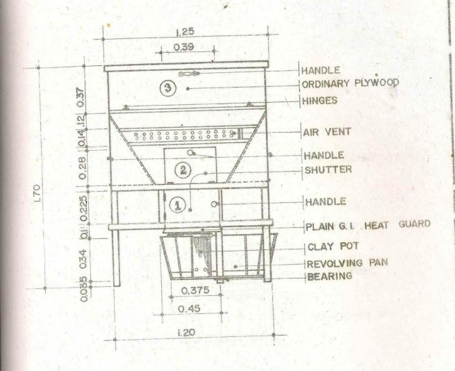
FIG. 3. FRONT ELEVATION Scale: 1:20 meter
