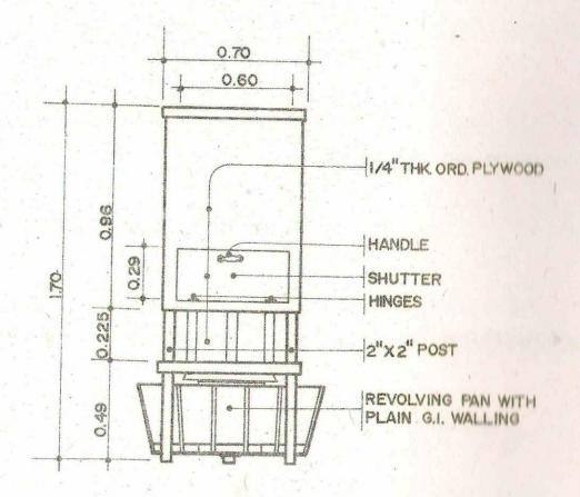
FIG. 5. LEFT SIDE ELEVATION Scale: 1:20 meter
