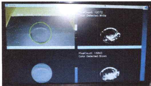
Figure 7. The monitor showing the feature extraction during the training phase
