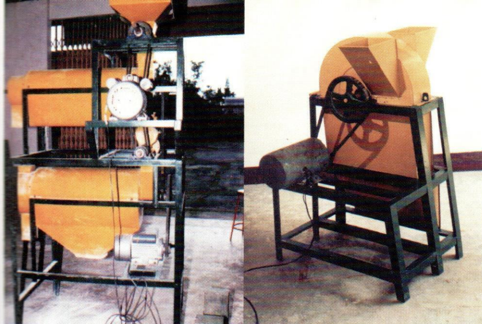
(Left) Micro flourmill for milling dried root crop chips; (Right) Grater chipper for root crops fabricated by the PhilRootcrops.
