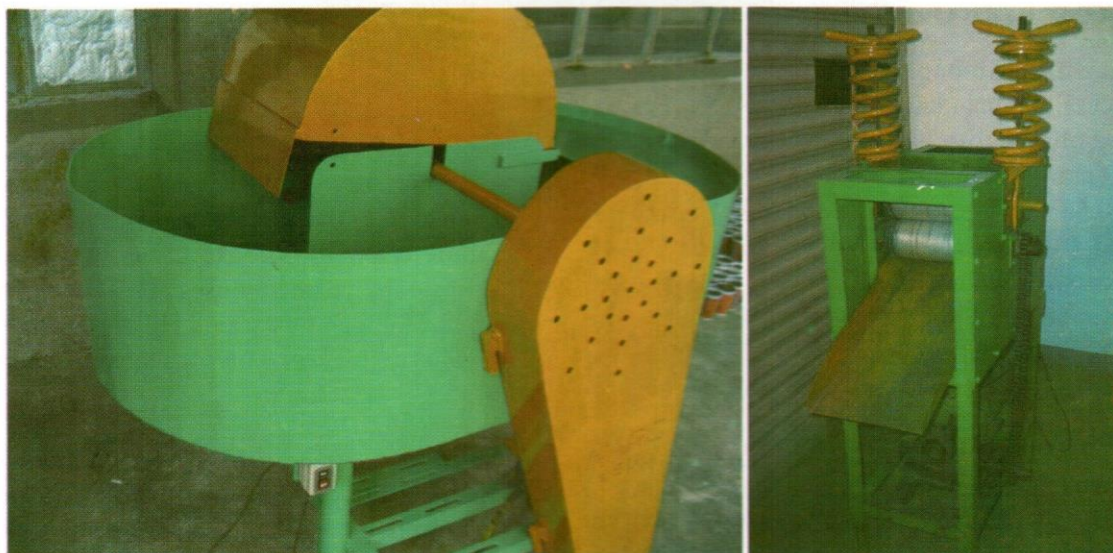
The improved abaca pulper and calendaring machine developed by the National Abaca Research Center..
