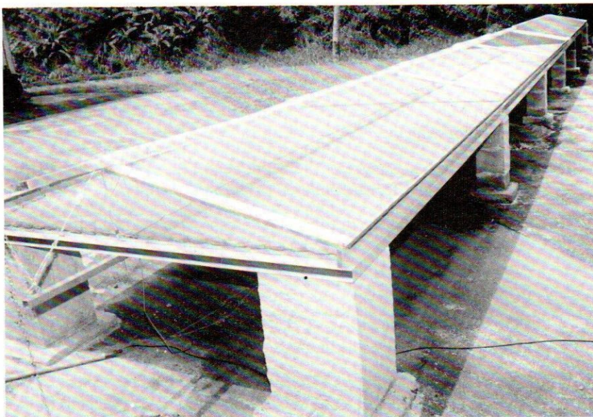
The Solar Tunnel Dryer donated by the University of Hohenheim, Germany.
