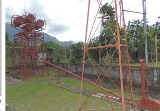
The Ram Pump Testing Rig showing its parts: water storage tank (1), stand for access valve (2), water header tank (3), and drive pipe (4)
